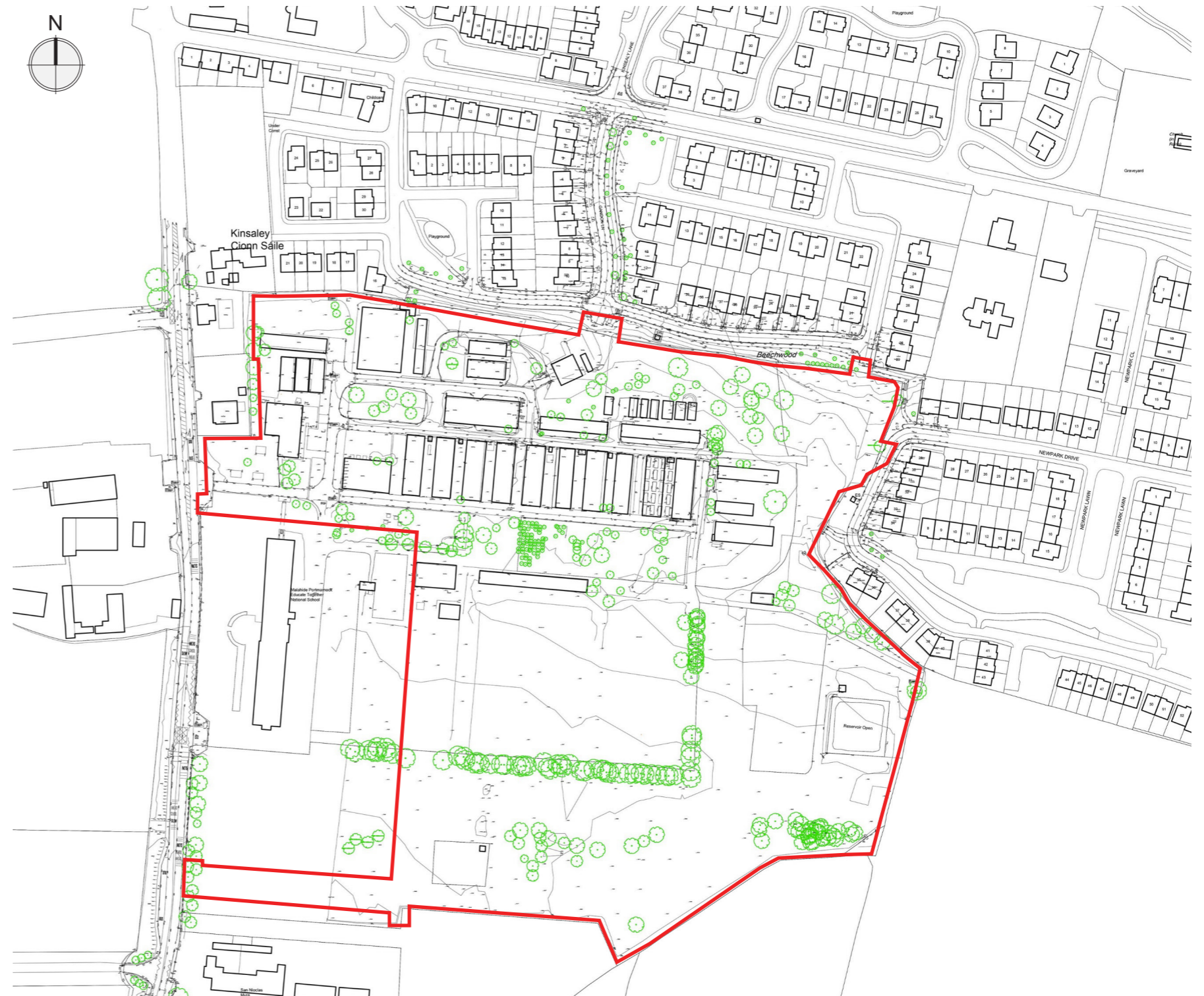
Figure 1.3 - Topographical survey of the existing site.
